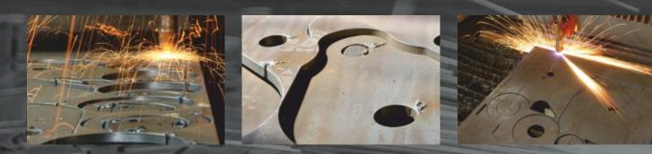
One of the latest plasma cutting solutions is the HD class: the acronym stands for two features, High Density plasma flux generators and High Definition of cutting provided by the plasma beam. The most important benefit of the HD-class technology is the minimum cut gap for precise fabrication of holes and sharp corners with a minimum edge profile chamfer which does not exceed 2%. This technology is good for cutting structural steel, stainless steel, acid-resistant steel and aluminium.
