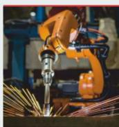
The welding fixture installed on a robotic manipulator helps weld all types of seams. The steady speed of stepless motions provide a high processing and finish quality of welds. The working range can be improved by deploying the robot on an additional linear motion axis.
