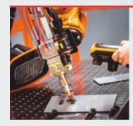
A plasma torch or a laser cutting head provides nearly limitless cutting applications. The excellent kinematic performance of industrial robots helps fabricate all types of welding chamfers and cutting of finished products, like shipping containers, ship's sides, and complete steel structures.
