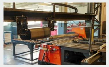
Uni-Kat designed and built an assembly line on custom order for production of large-diameter ventilation ducts for nuclear power plants. The processing line components include: a sheet metal loading station that handles workpieces up to 2000 x 6000 mm in size and 4 mm thick, a sheet mill station for cold-forming of sheet metal into a custom cross-sectional shape, a duct unloading station and a dedicated linear welding machine.
