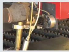
The dedicated design of the magnetic torch holder protects the torch upon impact against a protrusion or a warped workpiece feature. When the torch strikes an obstacle, the neodymium holder socket will release the torch to protect it from costly damage. The collision sensor is triggered at the same time to stop the machine without delay. The magnetic holder allows torch installation at an orientation of +/- 45°. This feature allows chamfering for downstream fusion welding operations.
